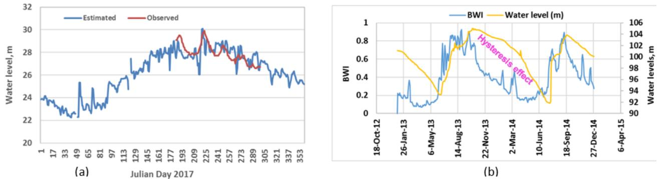
Figure 6: (a) Brahmaputra river (Dhubri) and (b) Reservoir (Ukai) water levels retrieved using Scatterometer datasets
