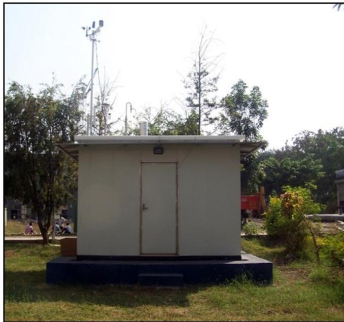
*Air quality monitoring station (AQMS) along with Automatic Weather Stations (AWS)*
