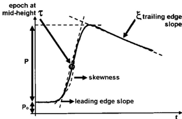
Figure 2: Power waveform from altimeter measurements
