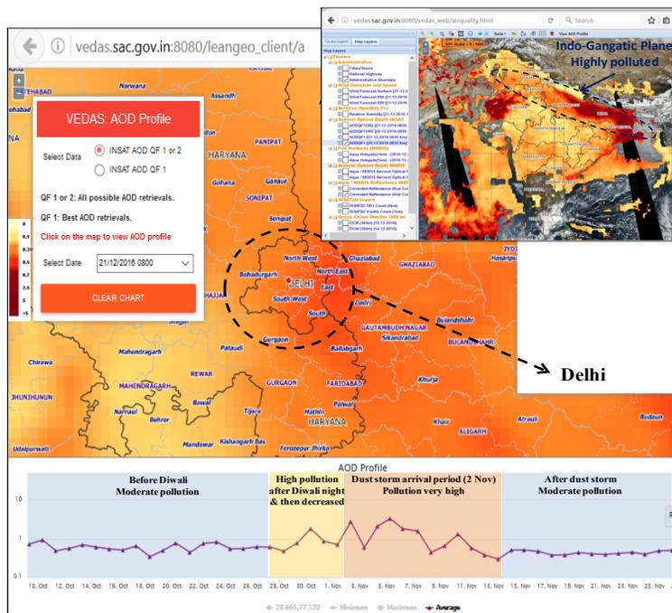
Figure 1: Snap shot of ISRO-VEDAS air quality web portal showing aerosol optical depth over Indian region. The temporal profile (at bottom) over Delhi region shows elevated air pollution due to the use of firecrackers for Diwali celebration (just after 28 October 2016)
