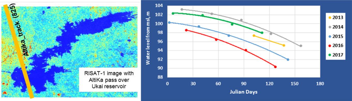
Figure 3: Ukai reservoir with Altika track and Altika retrieved reservoir water levels
