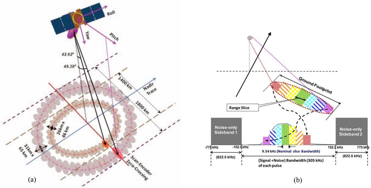
Figure 5: (a) Scanning geometry of OCEANSAT-2 and (b) partitioning of receiving bandwidth (source: Misra and Kumar, 2015; Misra et al., 2014)
