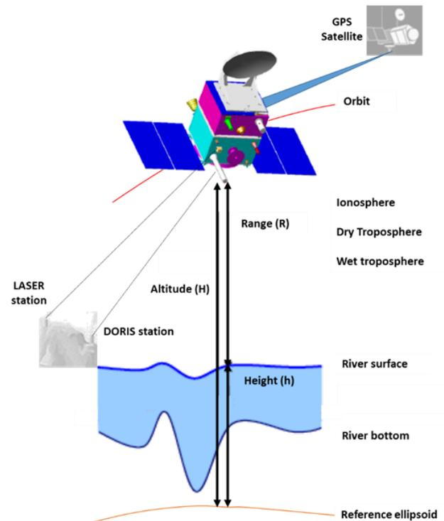
Figure 1: Altimeter principle of ranging
